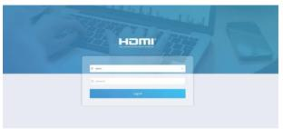
Select the initial username (admin) and input the initial password (1234) on the above login interface. Then, click "Log In" to enter the Web GUI interface. For the first time, you need to setup the project, as shown in the following figure:
