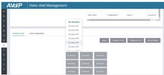
Note: A Decoder can only be assigned to one video wall.
