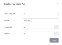
You can set the Video Wall ID, Name, Horizontal and Vertical panel numbers. Then click "Create" to create the Video Wall.
