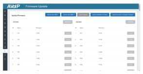
On this page, you can separately update the firmware of any Encoder/Decoder by clicking the corresponding "Update" button on the right, or update all the firmwares of Encoder/Decoder simultaneously by clicking the corresponding "Update All" button. Also you can update the Controller firmware by clicking
