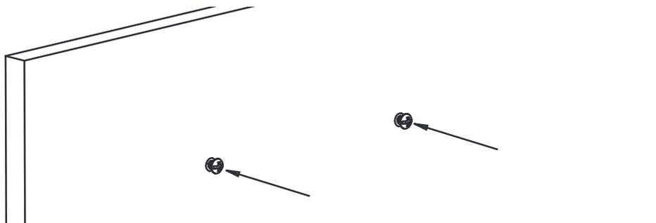
2. Hang the unit to the hanging hooks matching the bracket's hanger keyholes.
