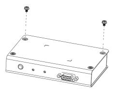
2. Use the screws you just removed to attach the mounting bracket that came with your package to the unit:
